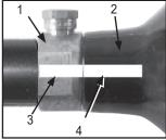
Properly marked Valve and Cylinder
