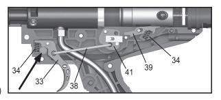
Trigger Adapter Assembly from the marker.
