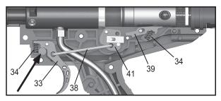
Trigger Adapter Assembly from the marker.
